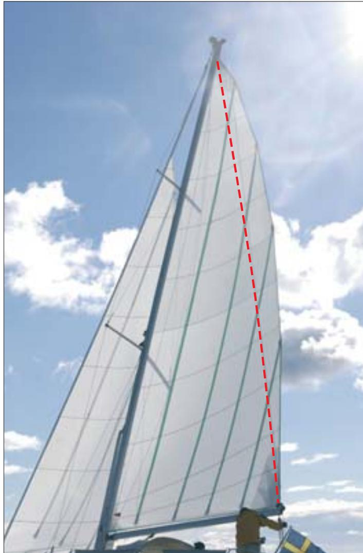
Anyone who imagines that a furling sail is less efficient because it cannot provide sufficient roach would be wrong. The new Seldén in-mast furling masts are made for vertical battens and a true positive roach.
