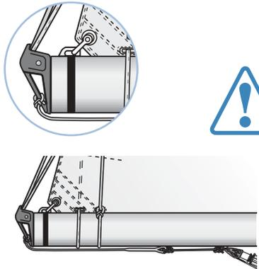
To facilitate the use of a preventer guy, a rope strop can be fitted permanently between the end fitting of the boom and the kicker slider. Tie the strop to the end fitting. The forward end has a spliced eye and a "guardrail" type lashing. When not in use, the lashing is tensioned to take up the slack.
