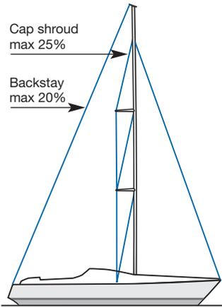
This type of rig is very demanding on the sailor, since it is complex to tune and to handle. In general, this type of rig needs more tension in the shrouds than a rig with in-line spreaders. The tension in the forestay is affected by three components;
