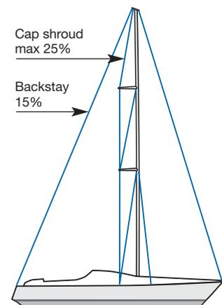
This type of rig is very demanding on the sailor, since it is complex to tune and to handle. In general, this type of rig needs more tension in the shrouds than a rig with in-line spreaders.
