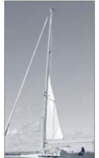
**Reefing;** we assume that the outhaul and furling line are led back to the cockpit, and that a rigid vang is fitted.
