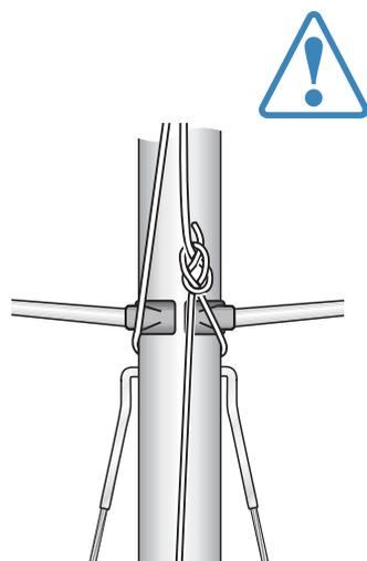
Make sure the strop does not interfere with the lower shroud attachments.
