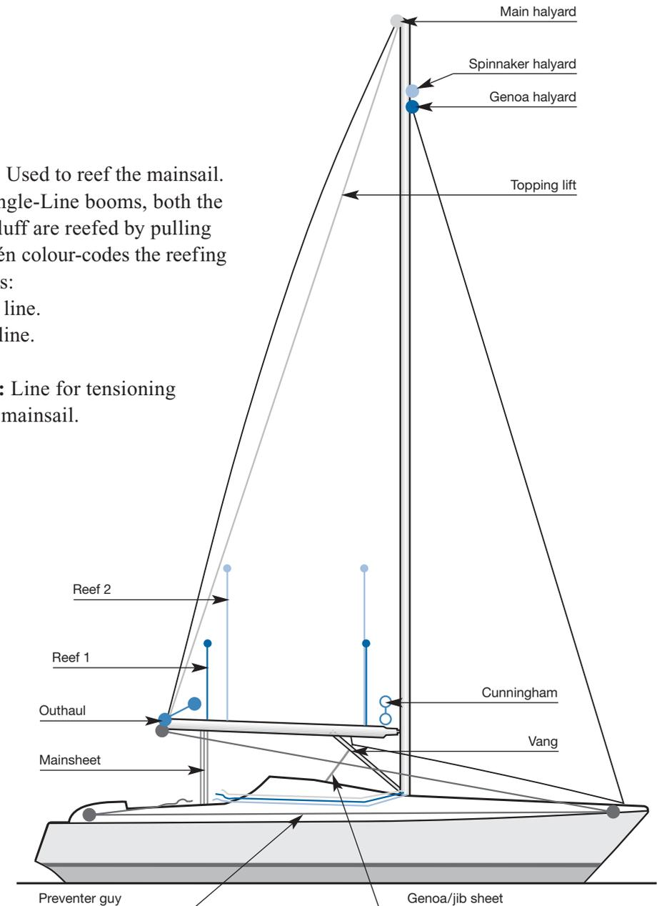
**Topping lift:** Used to prevent the boom end dropping into the cockpit when not supported by the sail, for example while reefing.
