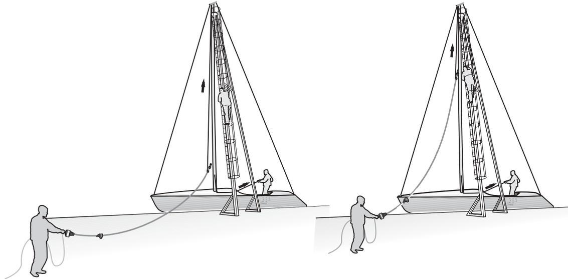
Normally, the jib furling system is placed on the forward side of the mast when the mast is being lifted by the crane. One person is detailed to prevent the system damaging the mast or yacht. The extrusion used in the furling system can cope with large radius bends without any problems, but may break in the event of uncontrolled buckling.
