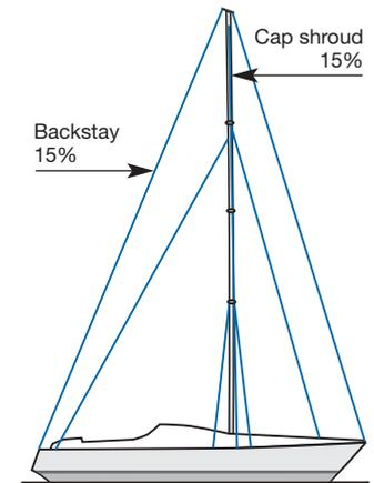
Continued: Masthead, multi-spreader rig, in-line spreaders, deck-stepped mast, forward and aft lower shrouds. Alternatively, baby stay and aft lower shrouds.
