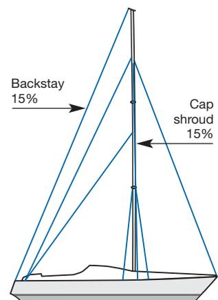
Runners are required to give sufficient longitudinal stability, and to obtain the required forestay tension. The backstays must be located as near the centre line of the hull as possible so as not to affect the lateral tuning. This type of rig is also found with single lower shrouds, in-line, and in that case checkstays are recommended to prevent excessive mast bend.
