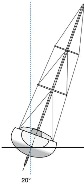
To ensure good fore-and-aft stability for this type of rig, it is very important that the leeward cap shroud is tight.
