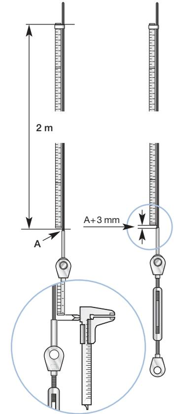
Hint! Count how many turns on the rigging screw corresponds to 1 mm elongation (5% of the breaking load). Make a note of it. This is useful to know if you ever need to tension “another 5%”.
