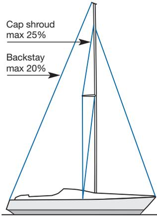
In general, this type of rig needs more tension in the shrouds than a rig with in-line spreaders. The tension in the forestay is affected by three components;
