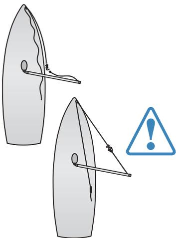
When connected, tension the bow line. Secure it to a bow cleat, or a cockpit cleat via a turning block.
